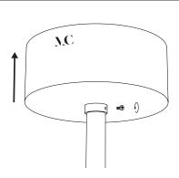
Pull up the thread guard after unscrewing the ring's screw.
