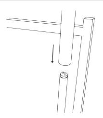
Put the opalin glass tube on the new neon tube.
