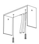
Fix the plate to the ceilling with dowels.
