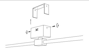
Unscrew the plate from the thread guard.
