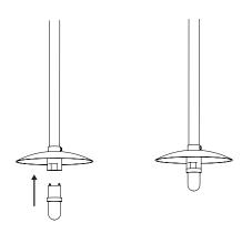
Insert the light source into the base.
