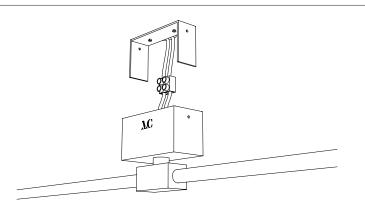
Connect the wires to the mains.
