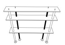
Place one of the trays in the 4 threaded rods of the 4 tubes A3, B3, C3 and D3.
