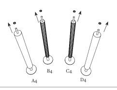
Unscrew the nuts on the threaded rods of the 4 tubes A4, B4, C4 and D4.
