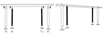
Place the 50 cm wide tray in the 4 threaded rods of the 4 tubes (A1, B1, C1 and D1).
