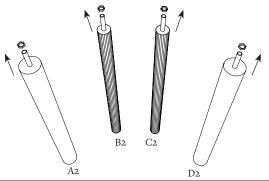
Unscrew the nut on the threaded rods of the 4 tubes A2, B2, C2 and D2. Note: the top of the tube is closed compared to the bottom of the tube, which is open!
