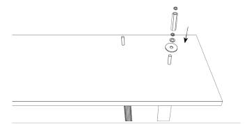
Assemble on the threaded rods of the 2 tubes A2 and D2 in this order: the large washer, the small washer, the nut and finally the coupling nut.
