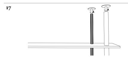
Screw on the upper part of the last tubes A4, B4, C4 and D4, turning until the plate touches the ceiling and the tube stops moving.
