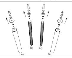
Unscrew the nut, 2 washers and coupling nut on the threaded rods of the 4 tubes A3, B3, C3 and D3.
