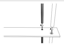
Insert the 4 threaded rods of the 4 rotating tubes A3, B3, C3 and D3 into the coupling nut fixed to the plate. tubes A3, D3 are on the outside and the splined tubes B3 and C3 are on the inside.
