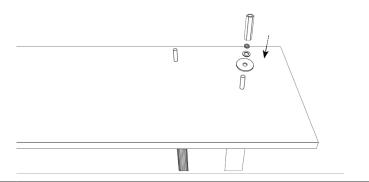
Assemble on the threaded rods of the 2 tubes A1 and D1 in this order: the large washer, the small washer, the nut and finally the coupling nut.
