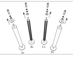
Unscrew the 2 washers, the nut and the coupling nut on the threaded rods of the 4 tubes (A1, B1, C1 and D1).
