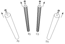
Unscrew the nuts on the threaded rods of the 4 tubes A3, B3, C3 and D3.
