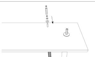
Assemble on the threaded rods of the 2 tubes B2 and C2 in this order: the medium washer, the small washer, the nut and finally the coupling nut.
