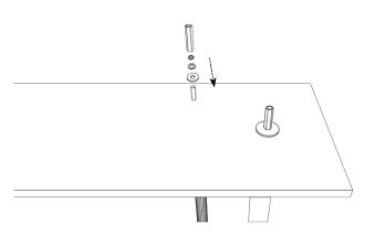
Assemble on the threaded rods of the 2 tubes B1 and C1 in this order: the medium washer, the small washer, the nut and finally the coupling nut.
