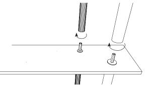
Insert the 4 threaded rods of the 4 rotating tubes A4, B4, C4 and D4 into the coupling nut fixed to the plate, with tubes A4 and D4 on the outside and splined tubes B4 and C4 on the inside.
