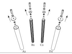
Unscrew the nut, 2 washers and coupling nut on the threaded rods of the 4 tubes A2, B2, C2 and D2.
