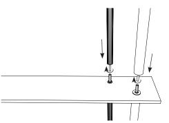
Insert the 4 threaded rods of the 4 rotating tubes A2, B2, C2 and D2 into the coupling nut fixed to the plate.tubes A2, D2 are on the outside and the splined tubes B2 and C2 are on the inside.note: pay attention to the direction of the tube, with the closed side facing upwards.
