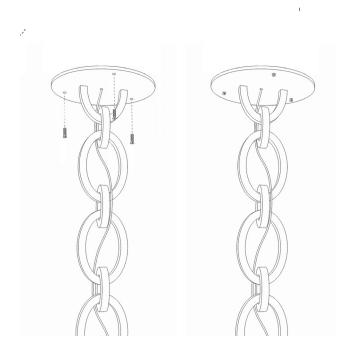
Refit the plate and secure it to the ceiling.
