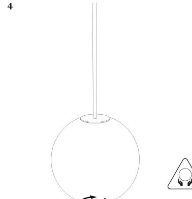
Screw on the glass globe, keeping the tube straight.
