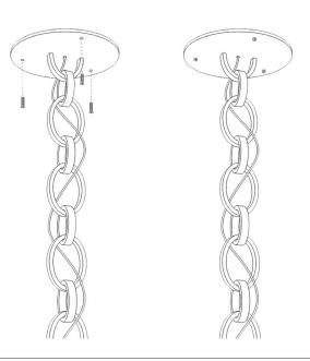
Refit the plate and secure it to the ceiling.
