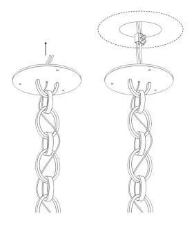
Connect the wires to the power supply.
