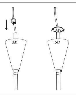
Take the ring previously unscrewed from the tube and pass the electrical cable through it, then screw the ring back onto the tube.
