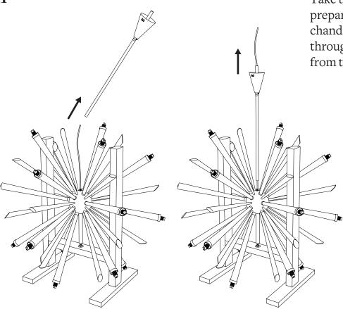
Take the tube and the canopy prepared earlier. Pass the chandelier's electrical cable through the tube and pull it out from the other side.
