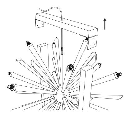
Carefully slide the top cleat off the trestle, guiding it along the electrical cable.
