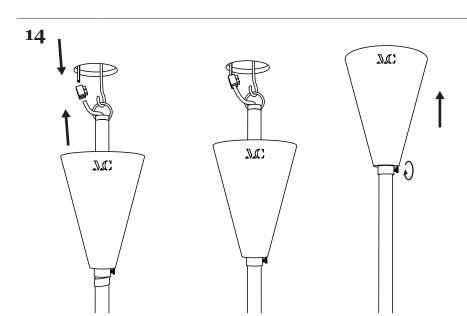
Keep holding the chandelier in the air while a third person installs the ring onto the hook in the ceiling.
