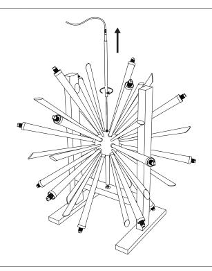
While the first person is still holding the chandelier, unscrew the small tube at the top of the chandelier, sliding it along the electrical cable.
