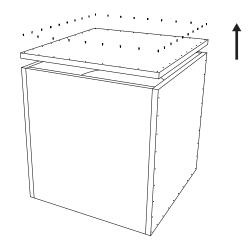
Remove the screws to take off the top plate of the wooden box.
