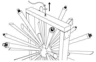
Remove the bolt and washer at the top of the trestle by sliding them along the electrical cable.
