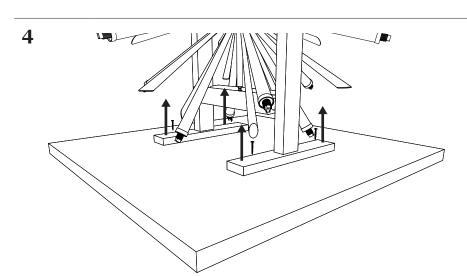
Remove the screws holding the two legs of the trestle to the bottom of the box.
