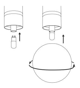
Insert the bulb into the socket. Screw the glass globe until resistance.
