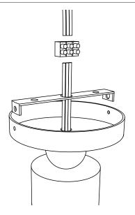
Connect the wires to the electrical network.
