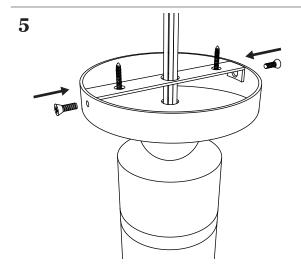
Place the ceiling light onto the mounting plate and secure it with the two screws.
