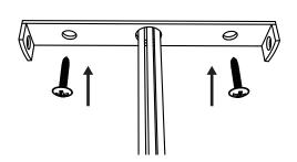
Position the mounting plate on the ceiling and fix it in place using the two screws.
