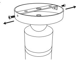
Unscrew the mounting plate from the canopy by removing the two screws.
