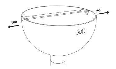
Unscrew the mounting plate from the canopy by removing the two screws.
