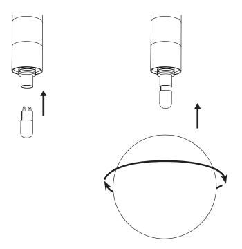
Insert the bulb into the socket. Screw the glass globe until resistance.
