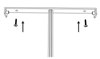
Position the mounting plate on the ceiling and fix it in place using the two screws.
