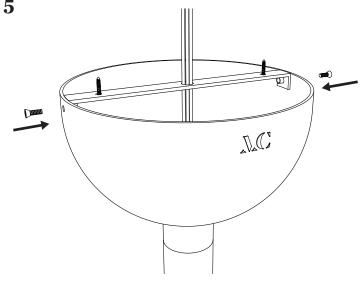
Place the pendant onto the mounting plate and secure it with the two screws.
