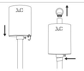
Loosen the screw on the ring slightly to lower the canopy. Place a piece of tape (such as painter's tape) under the ring to prevent the canopy from sliding down further.
