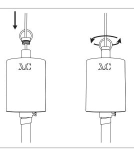
Take the ring previously unscrewed from the tube and pass the electrical cable through it, then screw the ring back onto the tube.
