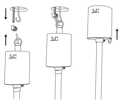
Connect the wires to the electrical network after installing the ring on the hook on the ceiling.
