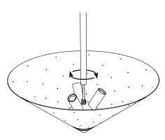
Screw the tube onto the reflector.
