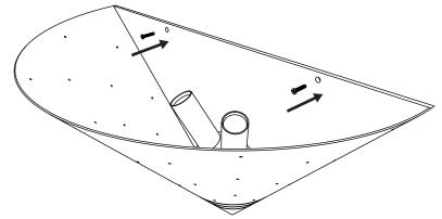
Position the wall light against the wall and secure it with the two screws.
